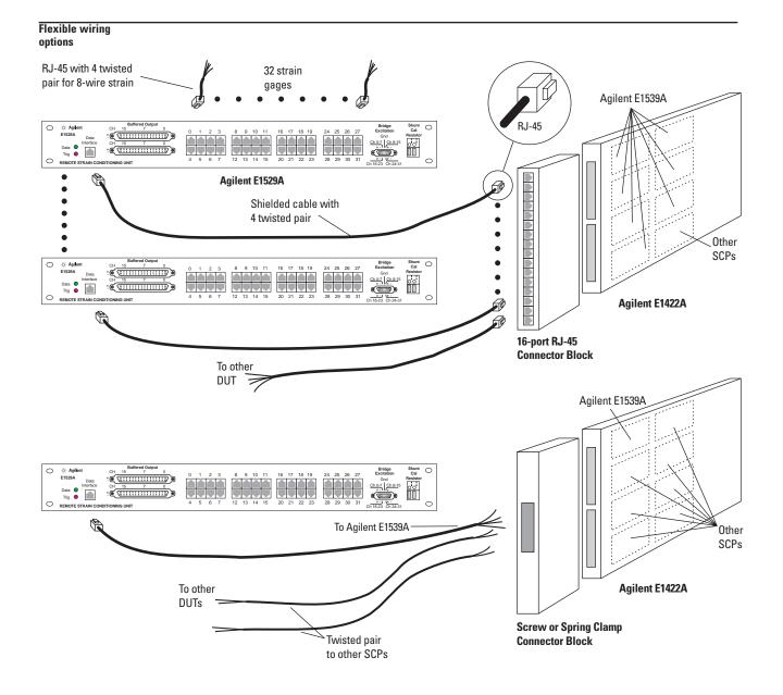
These accessories attach to the front panel of the E1422A and provide signal routing to the SCPs inside.
